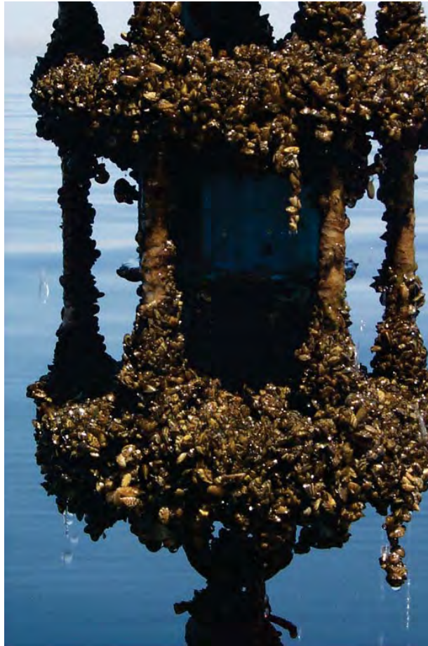
Figure 6.3: Retrieval of Zebra Mussel-Encrusted Vector Averaging Current Meter (Similar to an ADCP) 81
